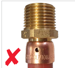
Witness hole not completely filled
