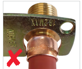
Fitting has been under crimped
