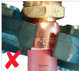
Jaw not square on the crimp ring
